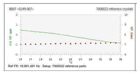
19,991,491 Hz FR: FL@20pf: 495.9 ppm C0: 5.4 pF 7.1 Ohms RR: C1: 25.2 fF L: 2.51 mH TS: 19.5 ppm/pF 0.21 Ohms DLD2: PWR: 109 uW 0.98 ' ANGL:
